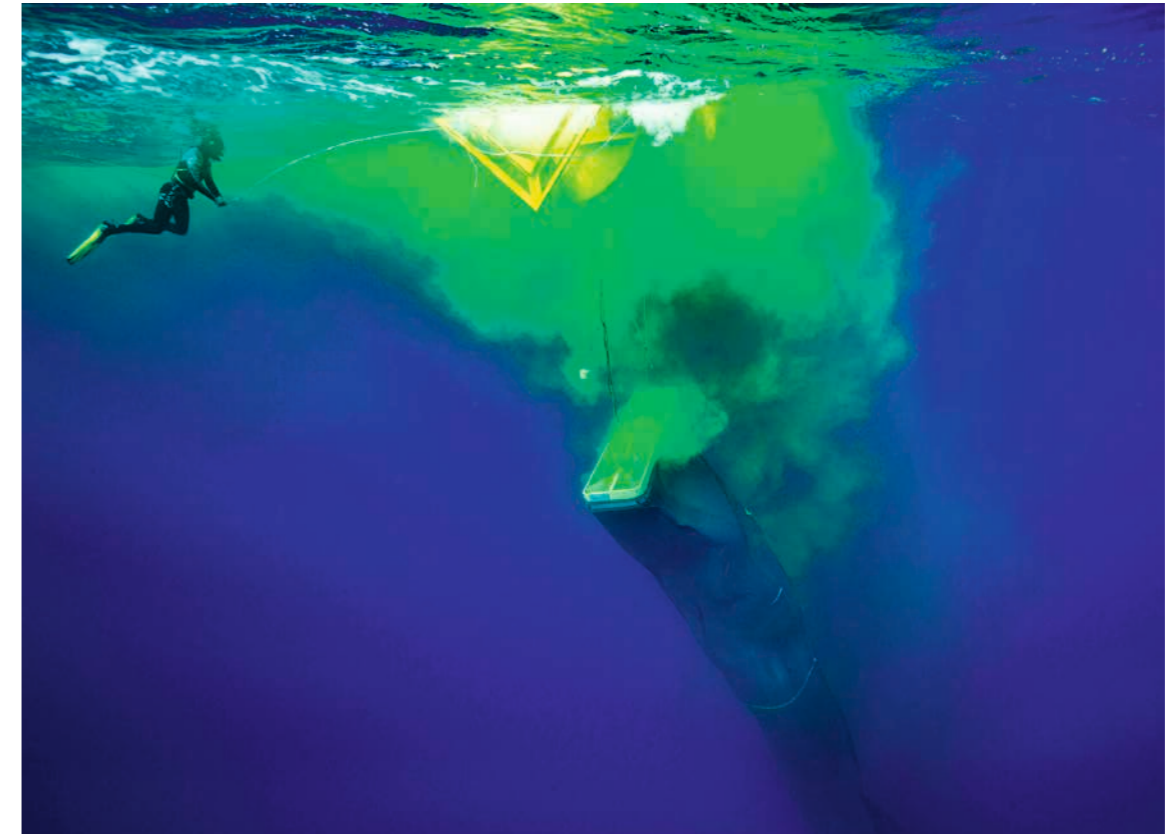
6.8 > In a wave pump test off Gran Canaria, the scientists poured a non-toxic bright green liquid made of seawater and the harmless fluorescent dye uranine into the upwelling tube in order to be able to observe how the deep water is distributed at the sea surface. Technical problems ultimately caused the experiment to fail.
