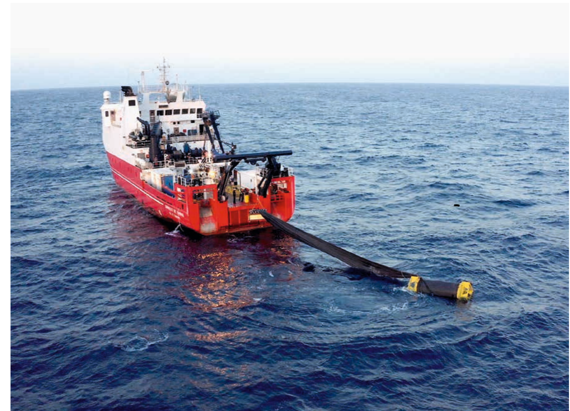
6.5 > The Spanish research vessel Sarmiento de Gamboa at sea with a wave pump. The pump was deployed in November 2022 for testing and research purposes in the Atlantic Ocean south of Gran Canaria. The dark upwelling tube is initially wrapped around the yellow buoy and only unrolls when the bottom weight drops down into the ocean depths.
