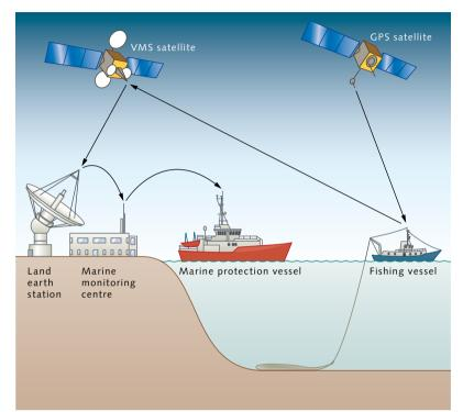
3.28 > Nowadays, fishing vessels must be equipped with electronic devices, or "blue boxes", which form part of the satellite-based vessel monitoring system (VMS). The blue box regularly sends data about the location of the vessel to the fisheries monitoring centre (FMC). Vessels are also equipped with GPS transmitters which track the ship's speed and position.
